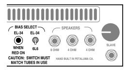
**NOTE:** It is extremely important that the **BIAS SWITCH** setting match the type of tubes in use. Failure to comply will result in damage to your amplifier. Always check the **BIAS SWITCH** whenever swapping tubes!
