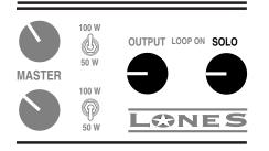
of a setting above that of the OUTPUT control and can not be set below. The amount of apparent boost also depends on that of the OUTPUT control - in that if the amplifier is at either the extreme low or extreme high levels of the OUTPUT, its effectiveness is minimized. It has been optimized for live performance volume levels.
