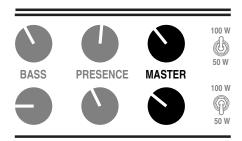
Again, we suggest using the **MASTER** control in its *sensible* ranges (9:00 - 2:00). Here, the channels will be easier to match with each other and the Effects Loop will see more reasonable signal levels.
