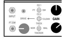
In most guitar amplifiers, and especially in all-tube circuits, the **GAIN** control is the most powerful control in the preamp. It shapes the overall style and character of the sound and is responsible for whether the sound is clean, overdriven or anywhere in between. In your **LONE STAR** the **GAIN** control is even more powerful. It not only determines the amount of drive, but also acts as an integral part of the tone control string as well.
