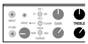
Like most of the controls on your **LONE STAR**, there is an optimum region of the **TREBLE** control where ample top end is mixed in and yet enough signal is still passed on to the MIDDLE and BASS controls.
