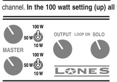
**100W / 50W: Channel Power Select:** These channel specific mini toggle switches allow you to preset the output power of each channel. **In the 100 watt setting (up) all four 6L6 are on line**, delivering maximum power and punch. **The 50 watt setting runs**
