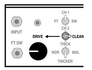
Set to CLEAN, all overdrive circuitry is removed and Channel 2 is a slightly higher gain clone of Channel 1. Because of this additional gain in what is otherwise a "rhythm" circuit, Channel 2 is an amazing solo channel for Roots style rhythm work or howling blues solo sounds. Cranking the GAIN control in Channel 2 CLEAN is a wonderful alternative to the more saturated sound of the **DRIVE** circuit.
